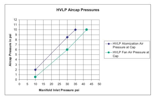
Fig. 1: HVLP Gun Air Cap Pressure
